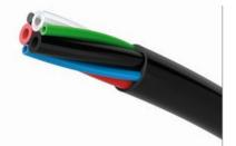
**SPEC 0083** 2 PLASTUB® PA tubes Ø4x6 + 3 PLASTUB® PA tubes Ø2.7x4 + 1 PLASCORD® 33 rod Ø6, assembled with PLASTUB® PVC33 black round sheath.
